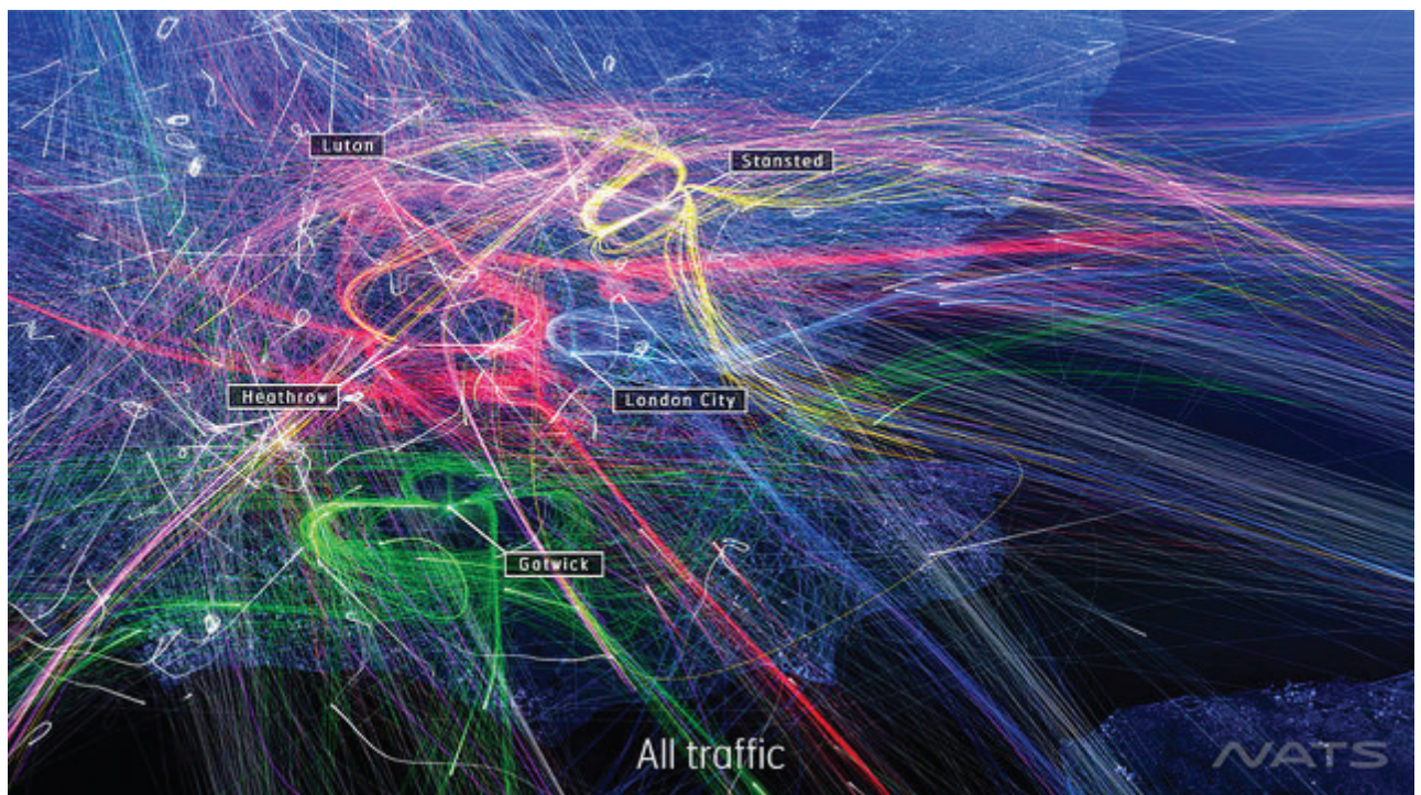
Figure 4.2 Radar tracks showing high levels of crossing traffic in today's London terminal airspace
